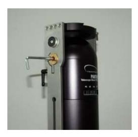
Release the two altitude clutch handles and rotate the counterweight arms to a horizontal position.
