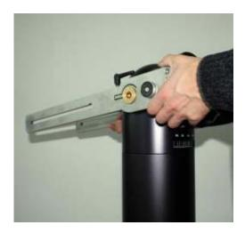
Remove the two brass axle adapters. They are conical in shape and locks a little in the end of the axle. To free them give the opposite side of the Top Mount Assembly a light blow with the hand.
